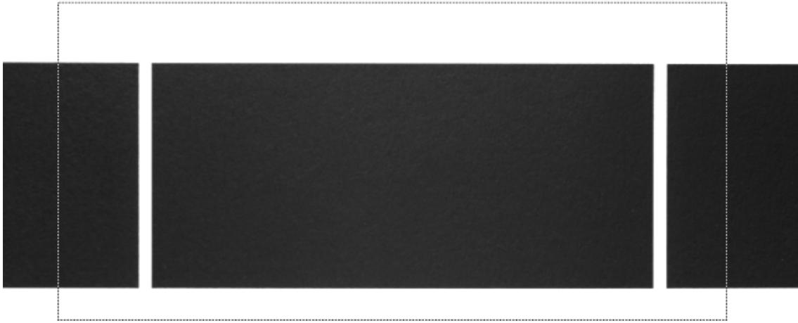
To define an AOI a left click on the mouse will enable a window to be drawn that reduces the image size both vertically and horizontally
