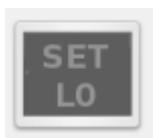
The Button SetL0 sets the actual length measurement as reference length L0 (initial gauge length). The strain measurement and the calibration are based on the reference length.
